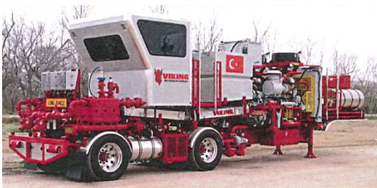
1200 Hydraulic Horsepower Trailer Mounted Twin Pump Acidizing Unit
